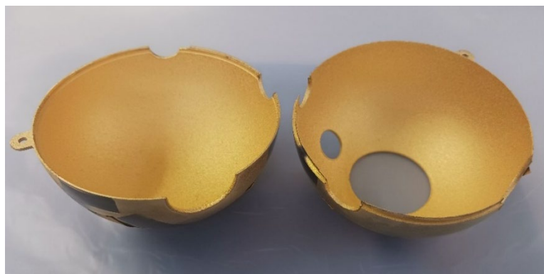
Figure 3: Gold-coating IR integrating sphere
