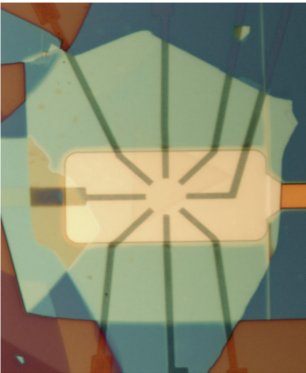
Figure 1: BN encapsulated WS 2 devices
