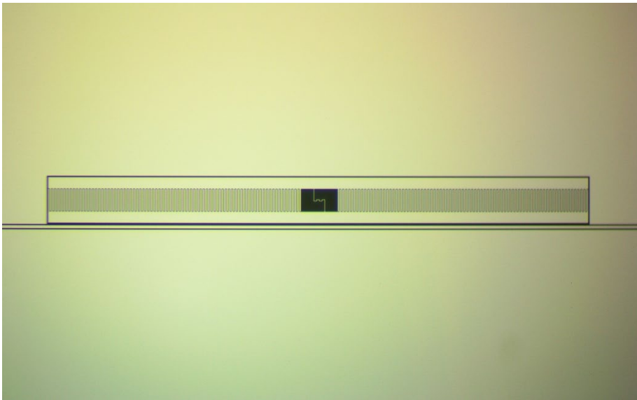
Figure 1: One Layer Nb lumped LC resonator coupled to CPW line.
